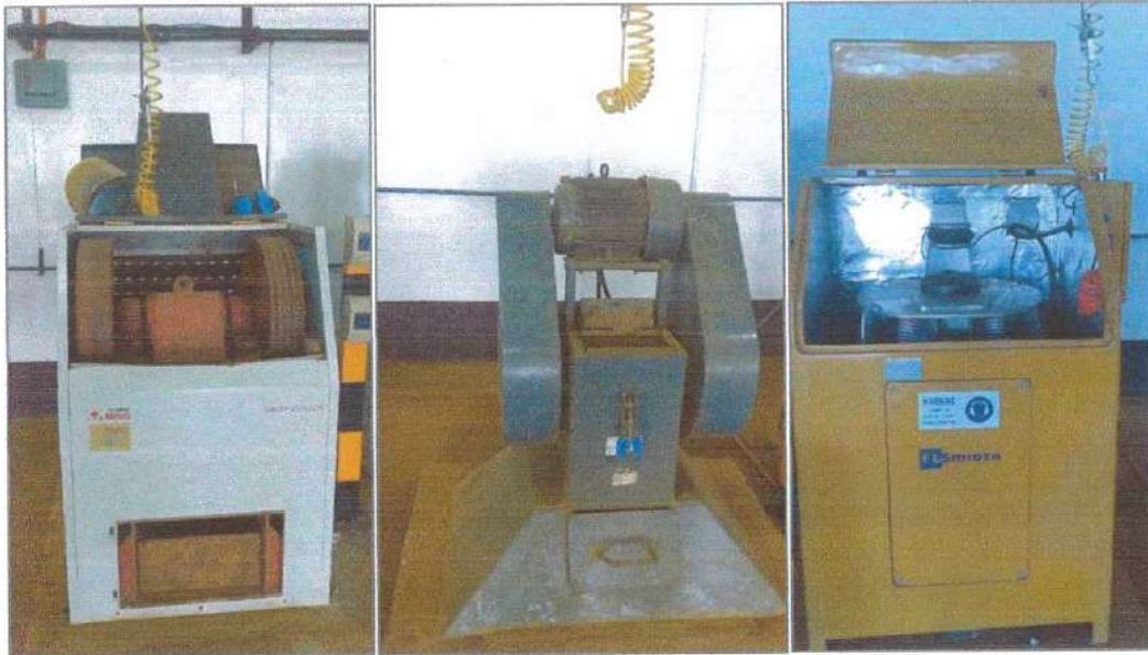
Figure 10-11. Primary jaw crusher, secondary jaw crusher and pulverizer.
