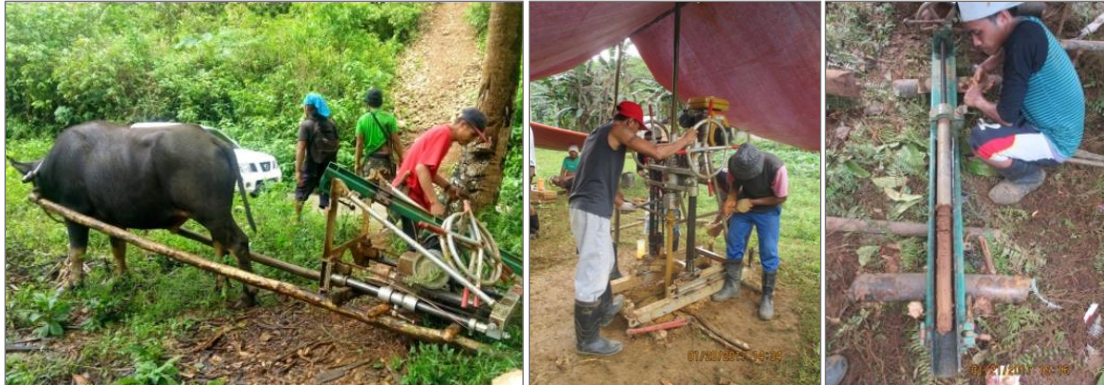
Figure 10-1. a) Mobilization of drill machine and accessories by manual hauling and at times using carabaos, b) actual drilling using YBM-YHP drilling machine, c) samples retrieval using core pusher.
