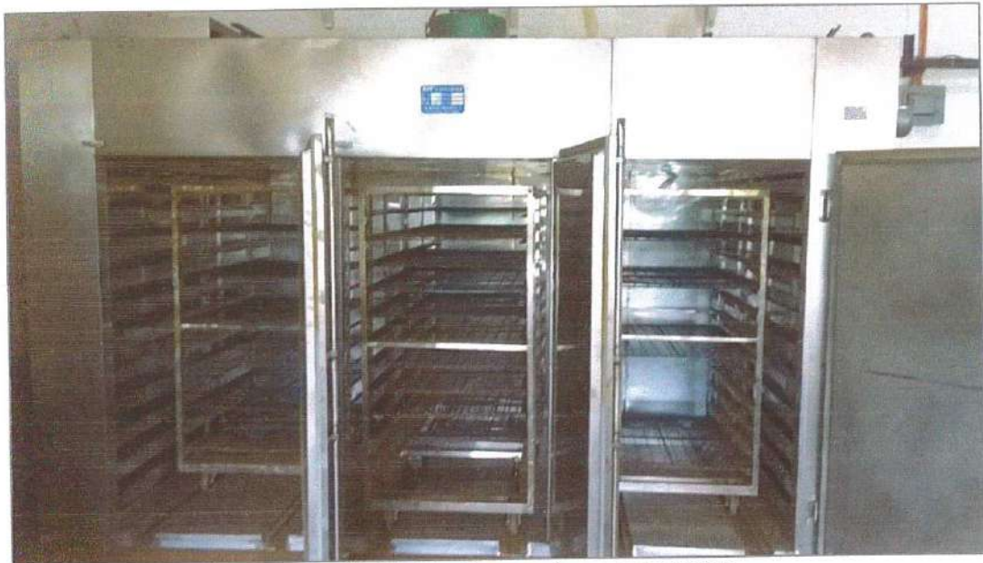
Figure 10-10. Electric oven for sample drying.
