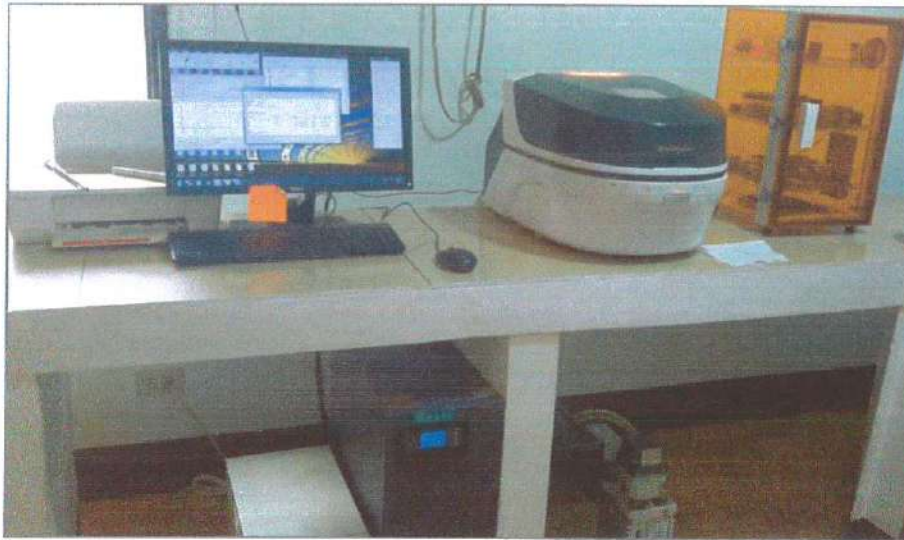
Figure 10-14. XRF-EDS Shimadzu brand with computer unit.
