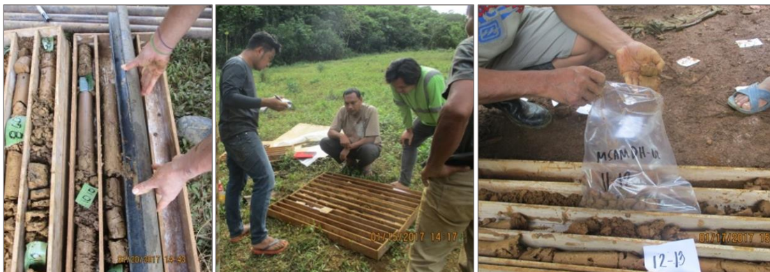
Figure 10-2. a) Transfer of sample from PVC pipe to core box, b) core logging of MMDC Geologists at field, c) transfer of samples from core box to plastic sample bags.
