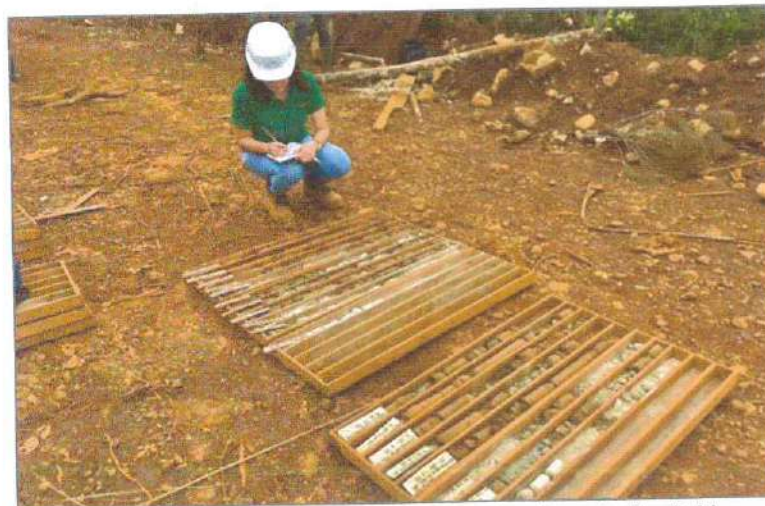
Figure 10-7. Core checking and logging done in the field.
